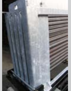
Corrosive protection, e.g. hot galvanised Box for drill rods
