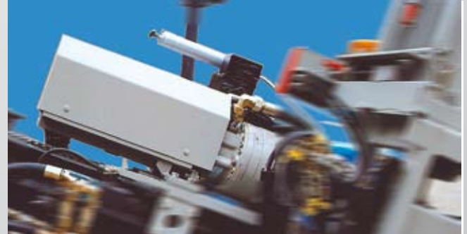
The percussive hammer works in even tougher soils, where other systems have to apply even more force.
