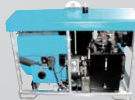
Hydraulic power unit TT M 9 for MA 09
