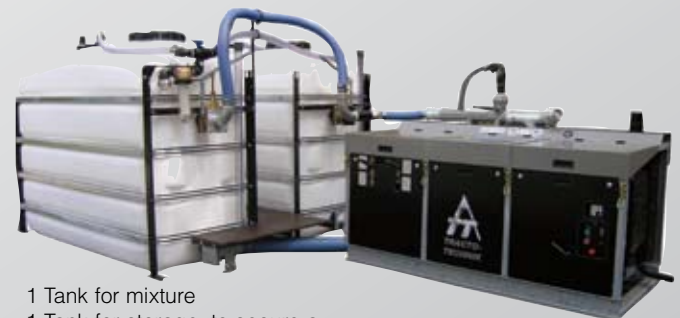
2 mixing tanks (2 x 1 m) each 4000 l
