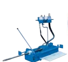
GRUNDOPIT - "P"-Family Models: Standard, Power, Shaft, Mini boring systems for pit launch 4 t pulling force, bores up to Ø 180 mm
