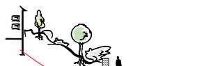
House connections underneath staircases, walls, slopes, in terrains which are not easily accessible
