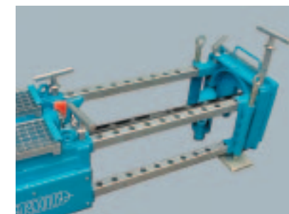
Adjustable telescopic support frame for safe alignment against the pit walls.
