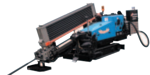
Grundodrill-HDD system, model: 7 X , with on-board mixing system DN ≤ 250, 200 m, thrust/pull back 65 kN
