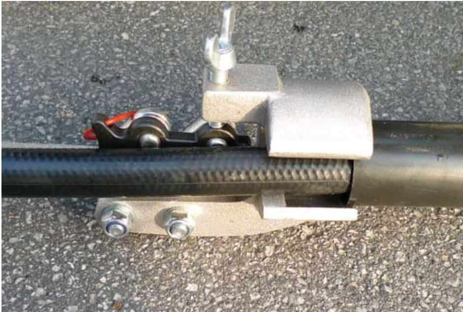
Pulling in accessories. e.g. for protection pipes.
