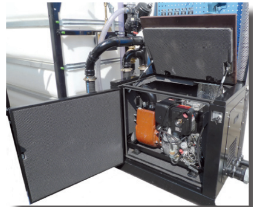
Practical and well insulated: The noise buffered drive unit with swing-up working surface.
