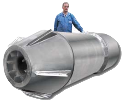
Long pipe expander ND 1060 with blade strips.
